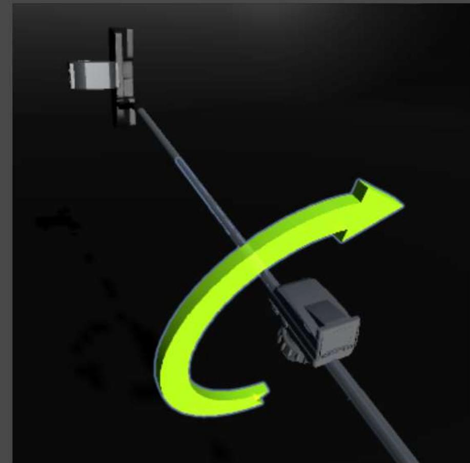
Rotate the Capto sensor as indicated until it is aligned. Fix it gently. Wait 3 seconds in position, the procedure is complete.
